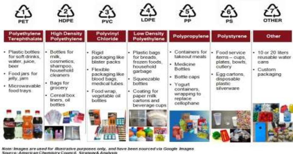
**Figure – 1: Different types of Plastic Packaging used in FMCG (Fast Moving Consumer Goods)**
